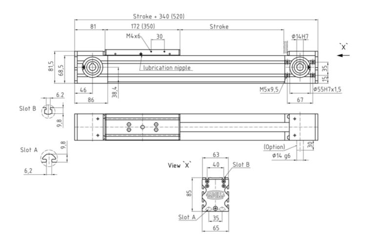
Stroke calculation: using distance and safety overrun Values in brackets for long carriage Motor connection see chapter Drive adaption
