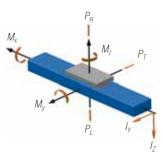
\* The dynamic load of the guide system is based on a nominal liftetime of 54000 km Values in brackets for execution with long carriage (254 mm)
