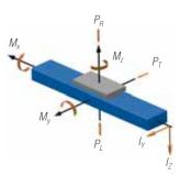
\* The dynamic load of the guide system is based on a nominal liftetime of 54000 km Values in brackets for execution with long carriage (580 mm)
