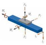
\* The dynamic load of the guide system is based on a nominal lifetime of 54000 km
