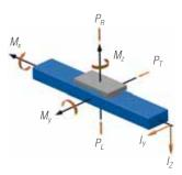
\* The dynamic load of the guide system is based on a nominal liftetime of 54000 km Values in brackets for execution with long carriage. Long carriage with rail guide upon request
