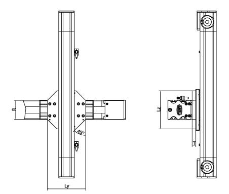
Centre of actuator = centre of carriage plate Adjustment using cylinder pins or stop angle
