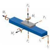
\* The dynamic load of the guide system is based on a nominal liftetime of 54000 km Values in brackets for execution with long carriage (460 mm)
